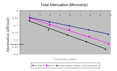
Insertion losses were measured using a ring resonator (1.88 mm trace width, 0.487 dielectric thickness, gap 0.15 mm, circumference 178.5 mm, internal radius 54.967 mm, external radius 58.727)
